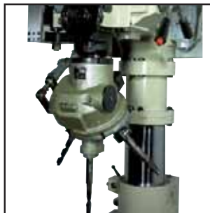
Cabezal múltiple revolver. Revolver multispindle headstock. Tête multibroche revolver. Mehrfachkopf, Typ Revolver.
