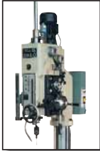
Roscador husillo patrón. Tapping system by lead screw. Filetage par vis mere. Leistspindel gewindeschneidesystem.
